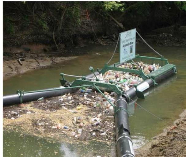
Bandalong Litter Trap in DC (*Stormwater Systems*)
